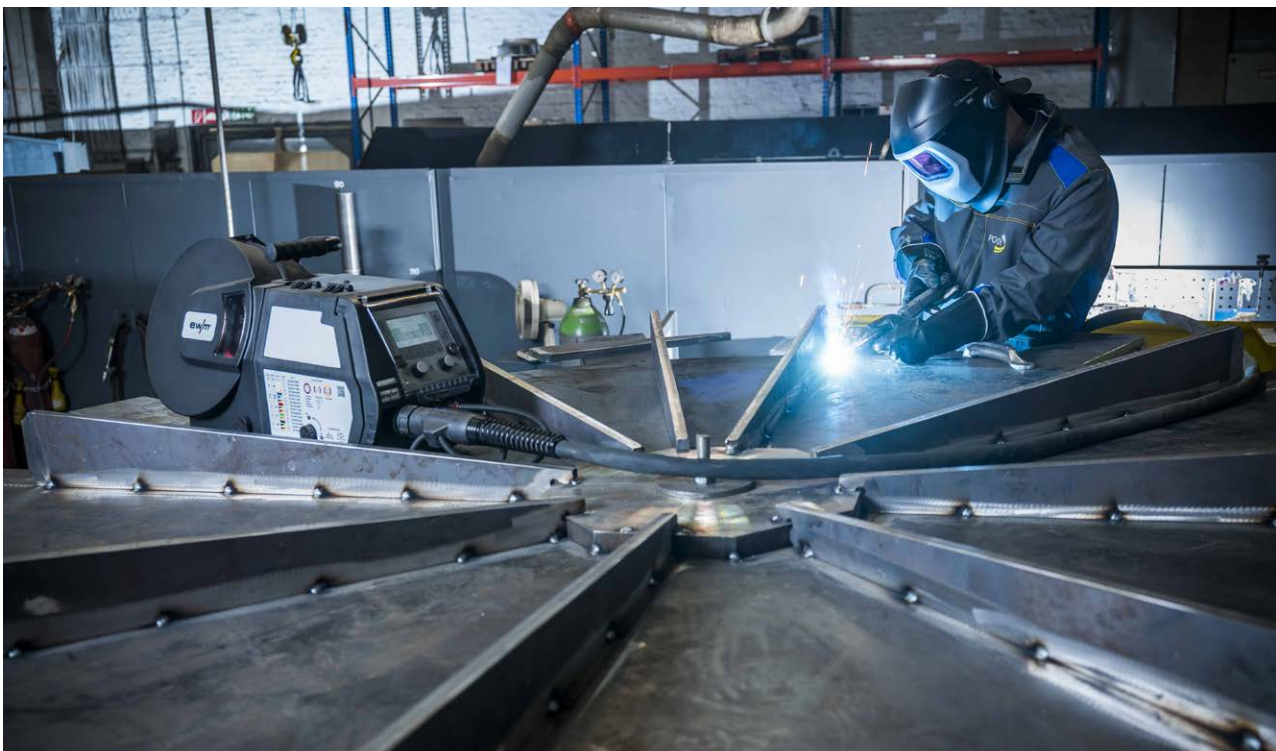
POLLRICH also designs and produces the tools for its own production. Here a faceplate for a pressure device is being reinforced with braces.
