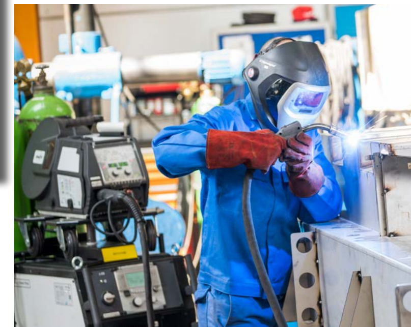
Virtually spatter-free welding of edge welds, fillet welds and butt welds on a nozzle casing of an annealing furnace. The low-heat coldArc procedure minimises distortion when joining the 2-mm-thick stainless sheet steel.
