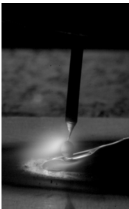
Droplet detachment after the pulse phase
