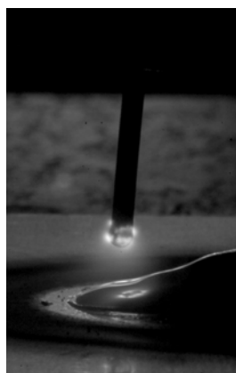
Cleaning and preheating of the wire in the negative phase
